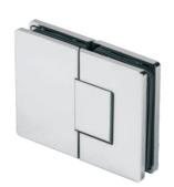
Spring shower hinge Glass thickness: 8-10mm Material: Brass Self Closing at about 30° Max.glass door weight 45kg/2 hinges
