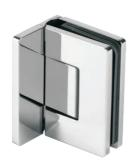
Spring shower hinge Glass thickness: 8-10mm Material: Brass Self Closing at about 30° Max.glass door weight 45kg/2 hinges
